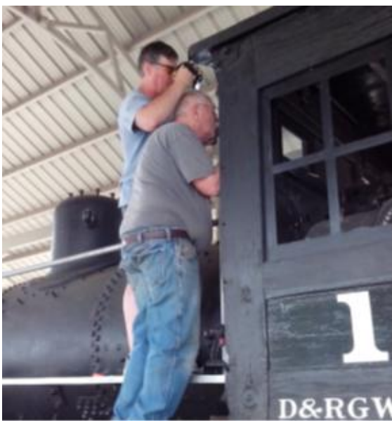
The Mendenhalls install one of the cab doors.
